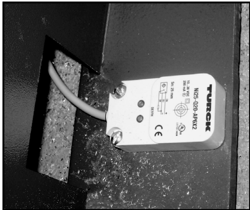
Figure 41 – Location of Upper Limit Switch, Control Cabinet
