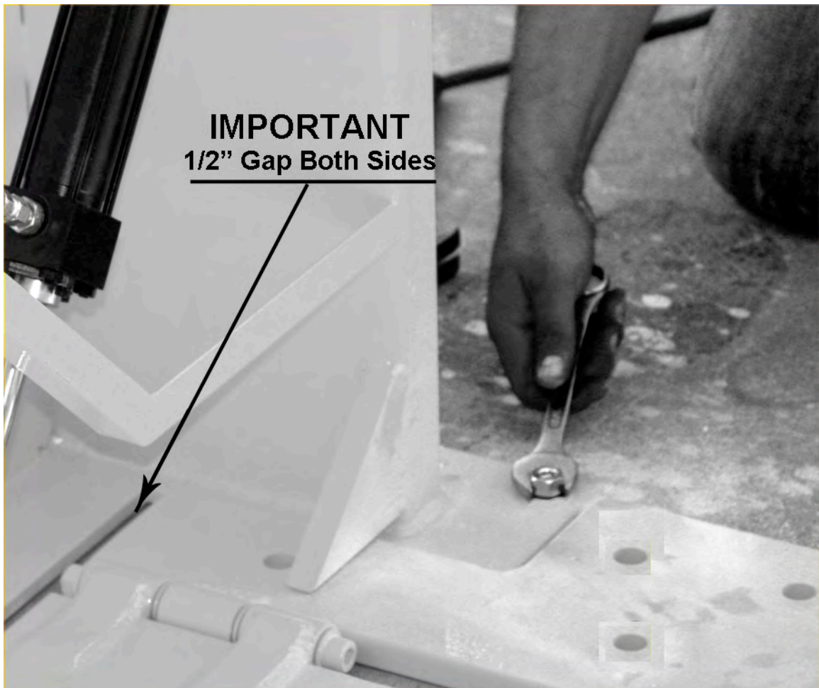
Figure 39 – Secure Anchors with Wrench for Final Attachment
