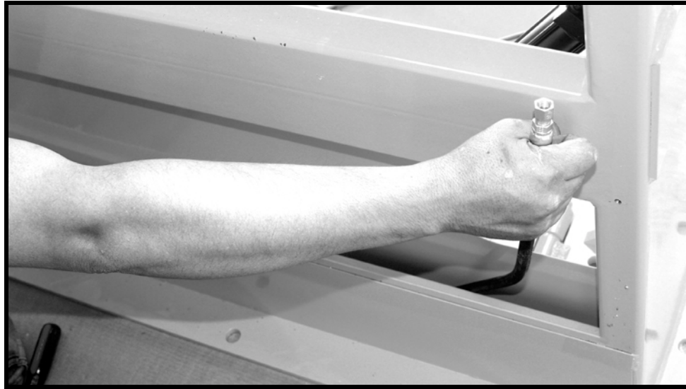
Figure 28 – Two Hoses Routed to Non-Control Cabinet
