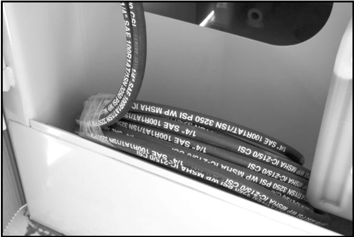
Figure 25 – Hydraulic Hose Location, As Shipped, Inside Control Cabinet
