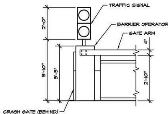
The figure above shows a Left Hand Control system with a traffic signal and OEM gate arm in front of the Spike System.
