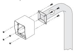
Using TEK screws, zip ties, or another type of fastener (not included), attach transceiver to inside wall or another surface of gate operator.
