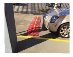
WARNING: Directional Traffic Spike Controllers are not intended to be used in areas where vehicular traffic is uncontrolled or crosses over the spikes at an angle other than 90°. Vehicle speed CAN NOT exceed 5 MPH. Speed Bumps and Warning Signs Must Be Used!
